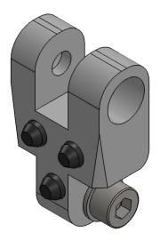
E865-T1-A - Extension piece for the top arm of the butt hook. Allows the arm to extend up and over the shoulder. Multiples can be added as required. Adds 26.5mm to length.
