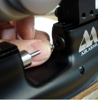
If the rifle does not cock, this may be due to incorrect trigger adjustment. The trigger also requires a pull through motion. If the trigger has not been 'pulled through' the sears may not have reset and will not be able to engage when the rifle is next cocked.
