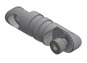
E865-B3-A - Extension piece for the bottom arm of the butt hook. Makes the arm longer and able to articulate. Multiples can be added as required. Adds 28.5mm to length.
