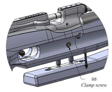
To adjust the cant and slope of the fore-end, loosen the three screws in the side of the clamp. It is best not to loosen the screws all the way as this will make it more difficult to hold the position of the fore-end. Once the desired position is achieved re-tighten the screws evenly until the clamp is secure.
