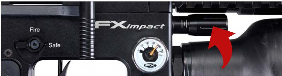
**2. Valve Control Knob** - The valve control knob is located between the barrel and the air bottle. Turning the knob CLOCKWISE will reduce the power, while COUNTER - CLOCKWISE will increase the power within margins. This adjuster will allow you to fine tune the valve flow and air efficiency. The default setting is near the center with 2 long lines and 2 short lines showing.
