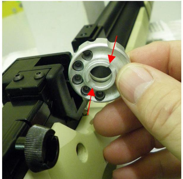
**Note:** To ensure the continued smooth operation of your magazine system, the pellet retaining O ring in the magazine needs to be regularly lubricated with a thin oil such as 3-in-1 to prevent premature wear and/or damage.
