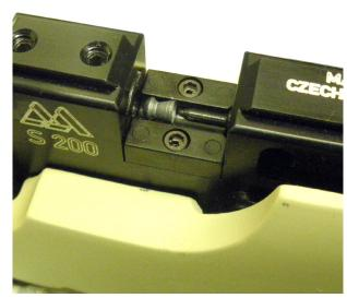
If you are using the pellet tray, when the bolt is in the rear position during the cocking cycle, place a pellet in the tray. When the bolt is closed it will push the pellet forward and into the breech ready to fire.
