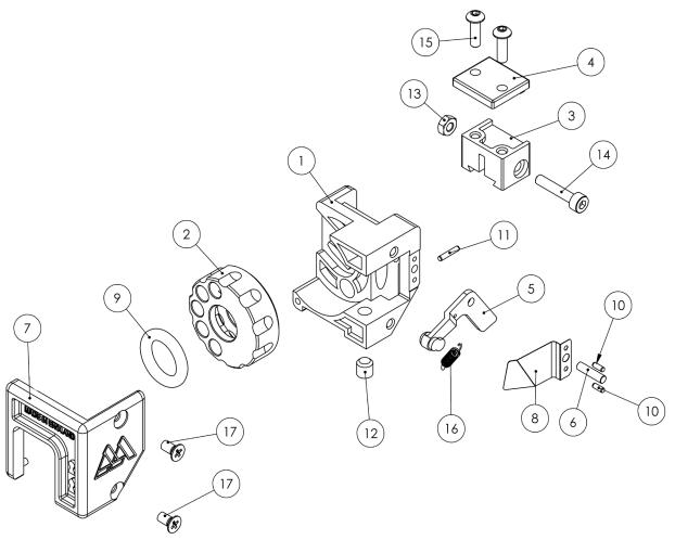
If you find that the magazine does not index correctly or the bolt will not go through, there is an adjustment screw on the left hand underside of the main body. This screw sets the position of the magazine and can be adjusted in (makes magazine rotate clockwise) or out (magazine will rotate anticlockwise). The screw has 2.5mm head and if you do make any adjustments, it is a good idea to make a note of them so you can return to the start position.
