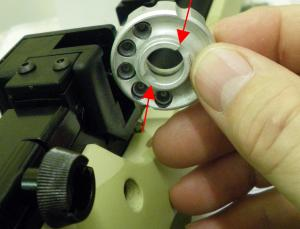
**Note:** To ensure the continued smooth operation of your magazine system, the pellet retaining O ring in the magazine needs to be regularly lubricated with a thin oil such as 3-in-1 to prevent premature wear and/or damage.
