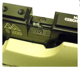
If you are using the pellet tray, when the bolt is in the rear position during the cocking cycle, place a pellet in the tray. When the bolt is closed it will push the pellet forward and into the breech ready to fire. If you are using a magazine system you will need to load the pellets into the pellet carrier.
