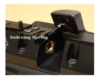
Be very careful not to damage the Indexing spring when demounting or mounting the magazine. Follow the instructions carefully.
