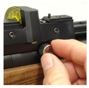
On the left hand side of the rifle is a indicator to help select your most common power settings + = High. - = Low. The marks do not indicate a particular power as this would change depending on the pellets used. The engraving maybe marked the other way round to the image below. This is normal and for manufacturing purposes.
