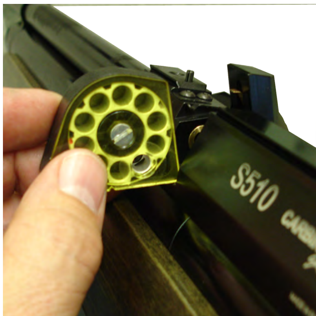
Pinch the magazine out of the housing
