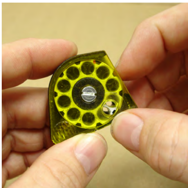
Manually turn the pellet carrier to the next empty chamber and load another pellet
