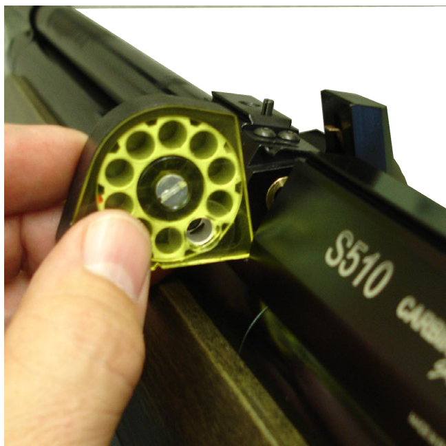
Pinch the magazine out of the housing
