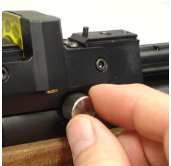
On the left hand side of the rifle is a indicator to help select your most common power settings + = High. - = Low. The marks do not indicate a particular power as this would change depending on the pellets used. The engraving maybe marked the other way round to the image below. This is normal and for manufacturing purposes.
