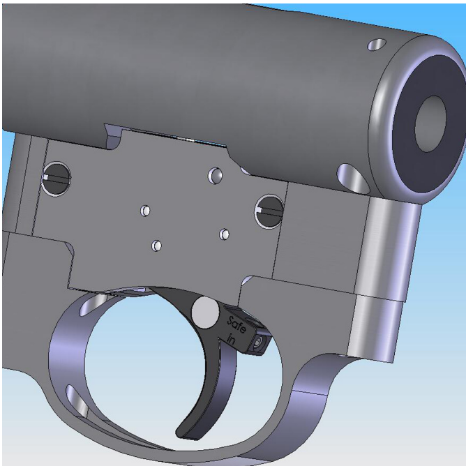
With the button pressed in the rifle is safe.
