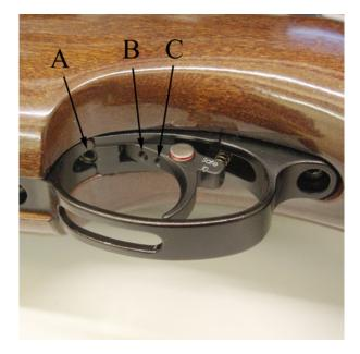
This rifle is fitted with a manual safety button located in the trigger blade. To make the rifle safe the button must be pressed until it is flush with the side of the trigger blade. Please note that it is possible to stop the safety button working with incorrect trigger adjustment.
