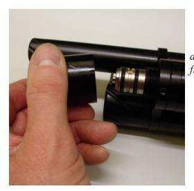
This is achieved by unscrewing the cover in an anti-clockwise direction. There is only one filling connector on the rifle and this fills both cylinders.
