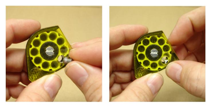
Hold the magazine and drop a pellet into the chamber. Manually index to the next empty chamber and repeat until the magazine is full. Finally line up the red dot on the pellet carrier with the 'V' notch on the clear magazine cover.
