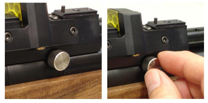
On the left hand side of the rifle is a indicator to help select your most common power settings + = High. - = Low. The marks do not indicate a particular power as this would change depending on the pellets used. The engraving may be marked the other way round to the image below. This is normal and for manufacturing purposes.
