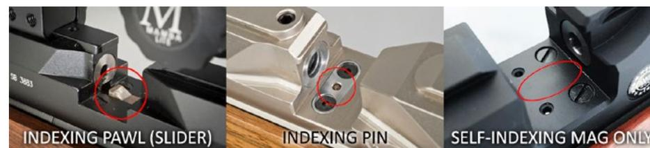
Fig 5: Breech indexing systems showing (from L-R) pawl, pin and no indexing mechanism. The latter style breech will only work with the Self-Indexing Magazine; the Self-Indexing Magazine may work in the other two breech types on older rifle models. The Multi-Shot Magazine will work in both pawl and pin breeches, but only if it is compatible and/or set up correctly for the specific rifle model
