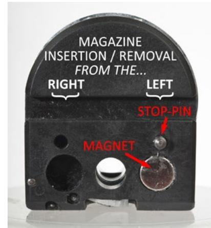
Fig 2: Double stop-pins (with magnet) to allow magazine to be inserted/extracted from right or left of breech
