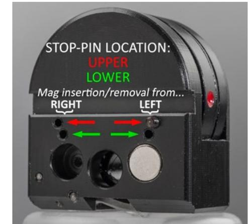
Fig 3: Additional upper and lower stop-pin positions for specific rifle models. Huntsman-style breeches require the lower position; breeches on the Pulsar, Renegade, Wolverine and RedWolf require the pin in the upper position
