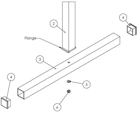
To fit the top bar to the uprights, slip the top bar (No.1) onto the M8 stud at the top of the upright assembly (No.2). The flange on the top of the upright must go left to right in line with the frame top bar assembly, also the hooks need to face front to back. Fix the bolt with a M8 nyloc nut and washer (No. 6 & 5). The bung (No. 4) can now be pushed into the end of the top member.
