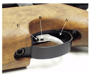
There are three adjusting screws. Screw (A) the weight of pull screw. This is under the rear of the trigger guard and the guard must be removed to make adjustments. Clockwise movement increase the weight. Screw (B) & (C) are in the trigger blade itself. Screw (B) adjusts the exact pull-off point. Clockwise decreases the pull-off point. Screw (C) adjusts the length of first stage travel, again clockwise decreases the length of first stage travel.
